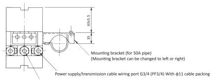
Electrode lead wiring port G3/4 (PF3/4F) with packing for φ8 lead wire
