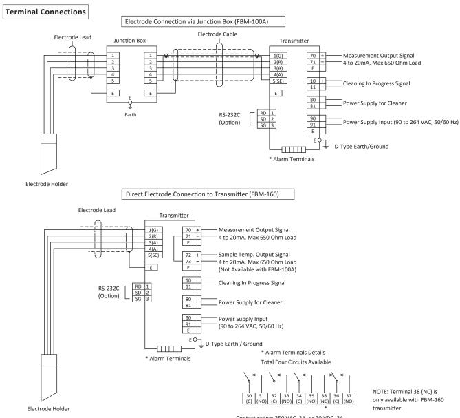
Contact rating: 250 VAC, 3A, or 30 VDC, 3A. Available Functions: high limit, low limit, under cleaning, under maintenance, meter error.
