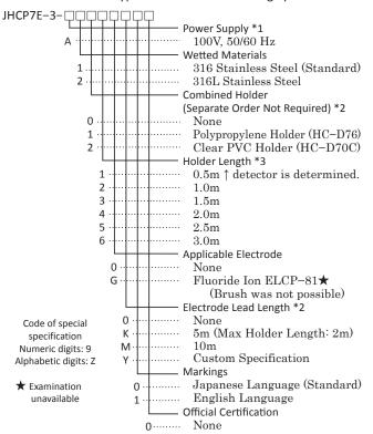
\*. Power Source fed to the detector via an FBM-type monitor. For Power Source greater than or equal to AC 100V, an antihypertensive trans (ZP:35VA) is required between the FBMtype and the detector. (Separately installed)
