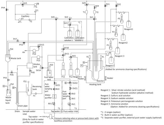
• 2 With flow path and external dilution device
