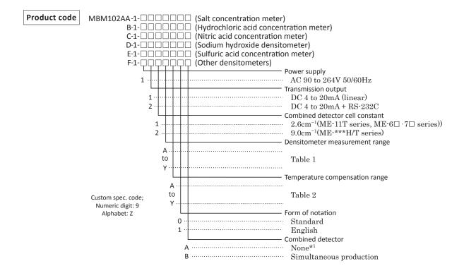
Note: The transmission output (4 to 20mA DC) is a linear output (linear) that corresponds to the concentration of the solution, so when upgrading from the MB-32 type (non-linear), it is necessary to change the scale of the receiver.
