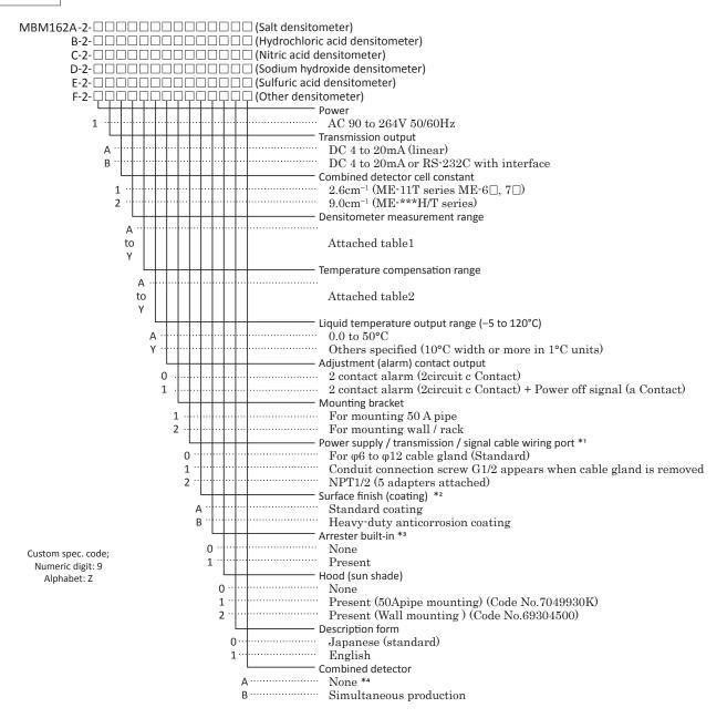
\*1. There are 6 wiring ports with  $\varphi$ 6 to  $\varphi$ 12 cable glands, but if you remove this cable gland, a wire pipe screw G1/2 appears.
