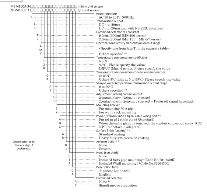
\*1. Other transmission output ranges can be arbitrarily specified with a width of 5/21 (23.8%) or more for each of the 7 measurement (display) ranges.
