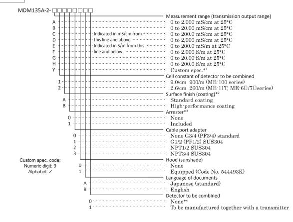
\*1. The measurement range can be freely reconfigured at a width of 25% or larger of each range. Example 1: When specifying a width of 25% for the 0 to 2.000mS/cm range – Please specify the
