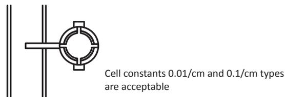
Figure B Vertical piping / horizontal mounting
