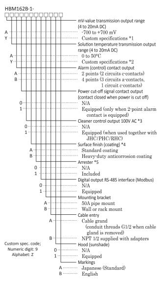
\*1. Specify the pH measurement output range in 0.01pH increments, with a minimum width of 2pH and a range of -1.00 to 15.00pH.
